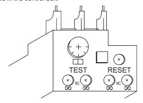
Figure 14. Over Current Relay
